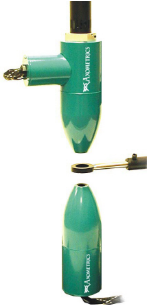
Figure 39 The Axoscan Mueller matrix spectropolarimeter is a flexible polarization characterization instrument.
