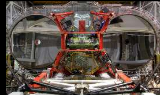
LBTI instrument (green structure) mounted between the two LBT primary mirrors
