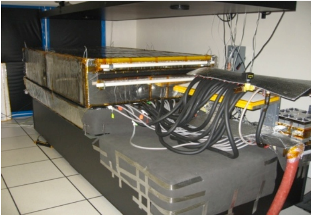
Figure 1: Actively stabilized thermal enclosure of the NASA Ames Coronagraph test bed.
