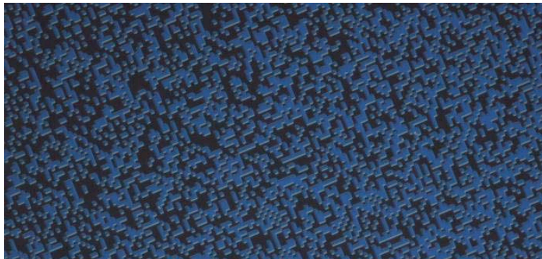
Figure 3-14: Half-tone apodizer using 2- \mu\text{m} black-chrome dots on glass (e-beam lithography). The apodizer is 12-mm diameter. (R. Soummer, STScI, A. Sivaramakrishnan, AMNH, and Daren Dillon, UCSC)
